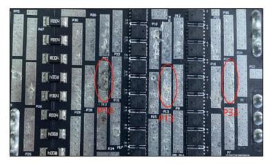
3) Measure the CHG and DSG test points on the mainboard without power-on. There should be no voltage. If there is voltage, the mainboard is faulty (or replace the mainboard for detection);
