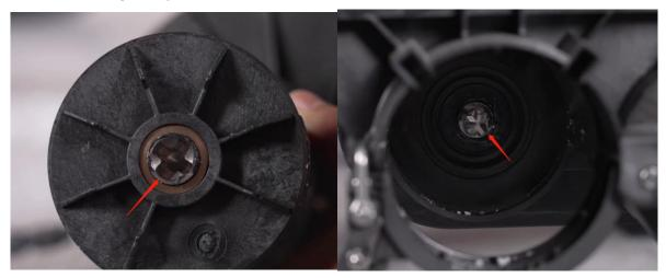
When placing the spiral feeder back to the slot, please make sure it follows the groove guide.
