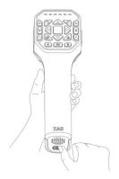
Optional: To eliminate the influence of 4G and make sure that ACS2 WIFI hotspot is enabled, we can **REMOVE** the SIM card
