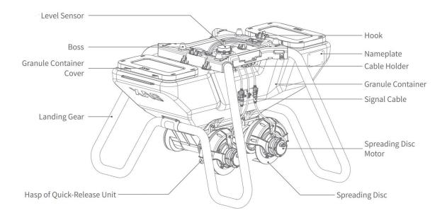
The two key mechanical parts of RevoCast system is the spiral feeder and spreading disc.
