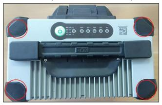
Step 2: Remove 4 screws from the upper shell of the smart battery
