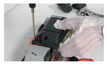
Step 2: Remove one screw on the positive and negative copper terminal.
