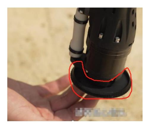
Check the RTK antenna installation
