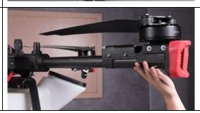
9. Inspect the joint of motors and base from loosening
