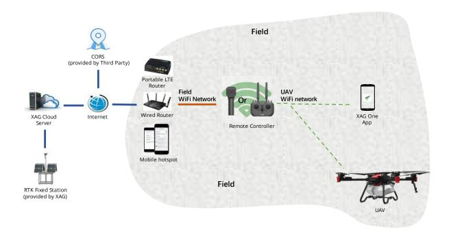
RCNWiFi - RTK portable station
