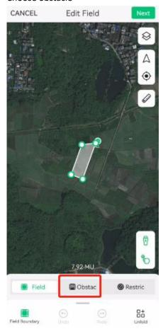
4. walk into the field and set points using ACS2 Rover. Press the 1st point to form obstacle
