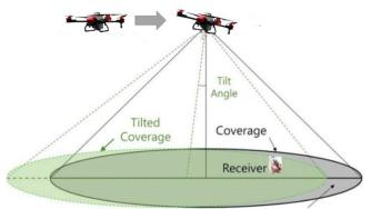
Shadow region in coverage made by UAV tilt
