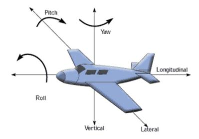
Angular measurement on the horizontal plane, with respect to true north, is referred to as yaw. Yaw is also known as azimuth or heading. The angular measurement on the vertical plane, with respect to the local level frame, is computed as pitch or roll.
