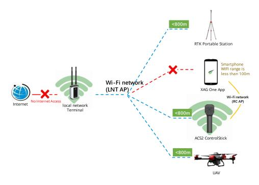
The benefit of this solution is that the communication range between smartphone and LNT increase from 100m to 800m in ideal environment. It's useful during field mapping, which the smartphone will be carried away from LNT.
