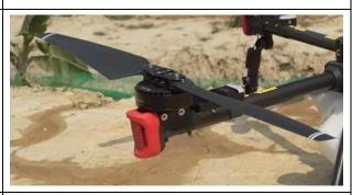
3. Inspect Airframe: Check the aircraft landing brace, arms, main beams to ensure there are no deformities, cracks, or breaks. Replace any unfit or broken parts. Inspect bolts attaching propeller arms to body. If bolts are loose use a sleeve to tighten the hexagon nut (recommended torque 20.0 kgf\*cm). If the tightening force is too small, replace the nut.
