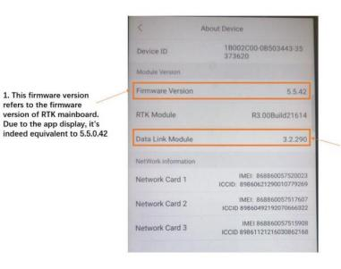
2. This refers to the firmware version of Data Link Module. Due to the app display, 3.2.290 is equivalent to 3.2.1.34, where 290-256=34.
