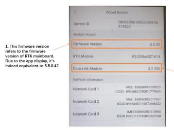
2. This refers to the firmware version of Data Link Module. Due to the app display, 3.2.290 is equivalent to 3.2.1.34, where 290-256=34.
