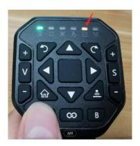
**b)** Make sure that the 5th LED indicator light become dim. If yes, your ACS2 remote controller has been reset successfully.
