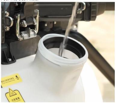
Emit the water from liquid tank to clean spray system again.
