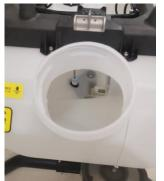
9. Check Charging System Connector: Inspect the charger and water tank plug (if using cooling tank) and ensure the plugs are clean and free of debris. Clean any debris and ensure all electrical plugs are dry before use.
