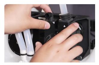
Inspect the lubrication between peristaltic pump internal rubber tube and plate synchronizer
