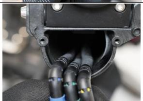
Inspect the cable connection of motors and ESCs from loosening.
