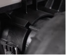
To lock the feeder easily, you are allowed to manually adjust the sprial feeder angle inside the container.
