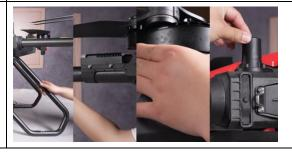
8. Inspect the rubber ring inside propeller clip. Replace rubber ring if it's worn out.
