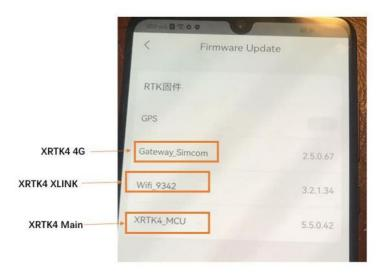
If your XRTK has the data link module is not 3.X.XXXX in XAG Agri2 or 3.X.X.XX in XAG One, then you will not able to use this method and have to use ACS2 2020 for XRTK firmware update.
