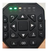
d. Turn on XRTK4, wait until the F1 light stops flashing and illuminate red.
