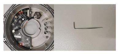
Note: The thermal conductive silicone pad pastes between the WIFI board and the bottom shield. It makes the WIFI board difficult to be removed from the bottom shell. In this case, we can use a heater to warm up the bottom shell for 1-~15 minutes. Then plug on the cable, grab the cable, and slowly pill the WIFI board away from the bottom shell
