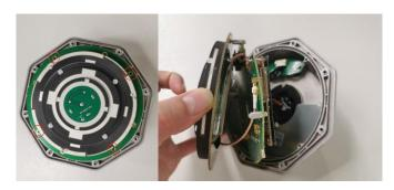
5. Unplug flexible flat cable and RF connector pins Please be aware of the aligning hole
