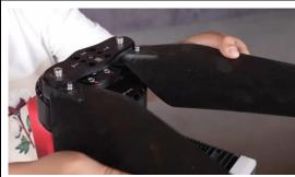
11. Inspect the screws (motor/clip) from missing or loosening
