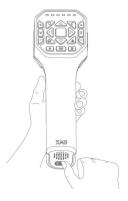
Wait 60 seconds until the ACS2 2021 completes initialization. Once completed, the third light indicator will stop flashing and becomes dim.
