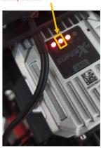
Flight control is connecting to internet through 4G as the 2<sup>nd</sup> light indicator (remote server) is in green.
