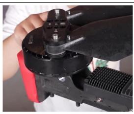
12. Inspect its bearings from loosening or abnormal sound. Rotate the motor to check the motor bearings
