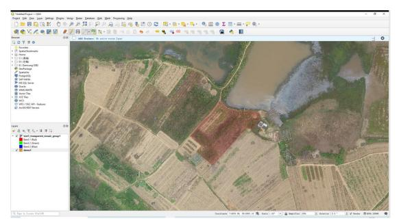
Fill out the fid, Name, type and description according to the feature attributes As we are drawing non-spray area here, the type must be "nospray"
