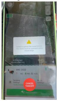
Analysis: The location is disabled. The app does not know the user's location. Thus, it fails the safety check because it can't calculate the distance between drone and user's smartphone. solution: enable the smartphone location feature.
