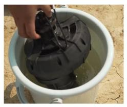
Use clean water to rinse spiral feeder. It's recommended to use high pressure water gun.
