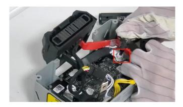
Step 3: Remove the battery plug
