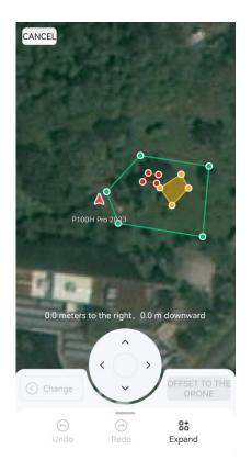
4. Select the target point (field boundary reference point), and then tap "Offset to the drone" button
