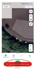
**Analysis** & **Solution**: This is due to the network connection delay. Please update the ACS2 firmware and the App software to the latest version, then try again.
