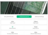
Advanced setting (Operation area, Follow terrain, Obstacle avoidance, Automatic route optimization for break point continues flight)
