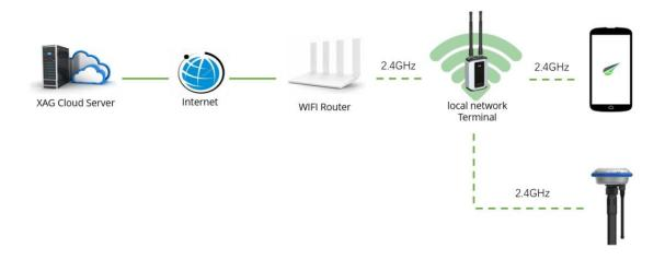
Please do not connect XRTK4 hotspot here. Because once XRTK4 WIFI access point configured, XRTK4 will automatically connect to LNT hotspot and XRTK hotspot will disappear.
