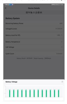
If you find battery balance lost (greater than 150 mV). Please turn off the battery immediately and move this battery to a safe place. Leave the battery alone for a few days and check if the cells can recover. If it can't, the battery may be scrap. Please contact XAG technician.
