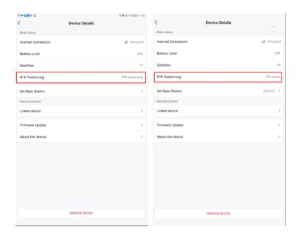
If the RTK positioning status is displayed as "RTK not connected" or "RTK positioning", ACS2 field mapping will not work. Make sure the RTK positioning status must be "RTK Active".
