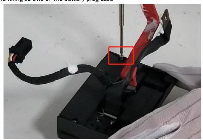
Step 2: Remove the battery plug case
