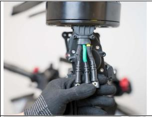
3. Inspect if the cables are intertwined or worn out (crackles, flaw, damaged, etc).
