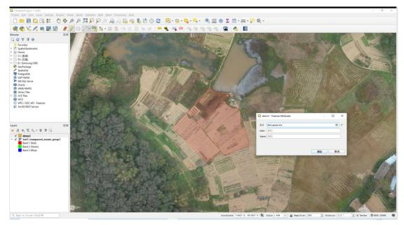
Fill out the fid, Name, type and description according to the feature attributes As we are drawing the field boundary, the type must be "boundary".
