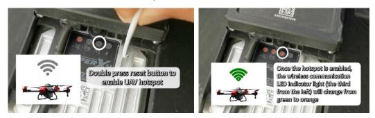
**Scenario**: double press reset button; the wireless communication light does not change to orange.
