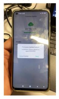
**Analysis**: This error could be caused by significant network latency. The XAG server is based in China, thus the user who are far from China, will evitable suffered from this.
