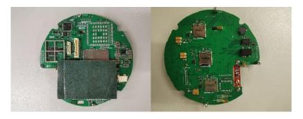
7. Separate RTK board and main board, unscrew 2 screws
