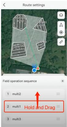
8 After setting flight routes, return to the operation interface by tapping the "<" symbol on the top left corner, Here you can set the spraying parameters.
