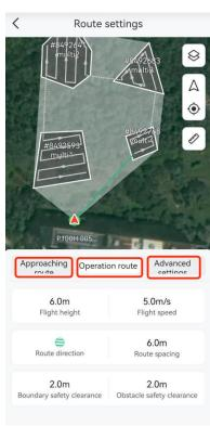
On Approaching Route setting page, you can set the speed, height, tap the entering route, "+" symbols will appear in the middle of each connection routes between the fields to enable you to set guide points for safe flight between fields.
