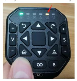
To test it, search the ACS2's WIFI hotspot under smartphone WLAN setting. If ACS2 hotspot can be found, it means that ACS2 remote controller has WIFI enabled and successfully switched from LNT networking mode to 4G.
