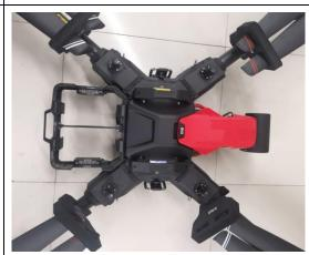
Screw inspection: Use a screwdriver and Allen key to check whether any fixing screws of the fuselage are loose, slippery, rusted or broken, and replace any damaged screws.
