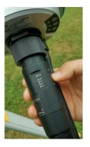
7. Insert XRTK4 into the tripod fixture slot, lock the clamp
