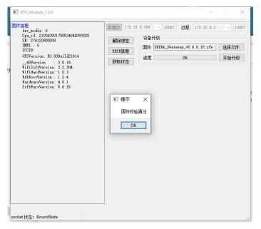
9. Click the button 开始升级 (start update), and there will be a progress bar prompt during the upgrade period, indicating the upgrade process. When the XRTK receives the firmware, F3 will flash blue, and when the upgrade is complete, it will beep twice。
