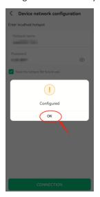
the prompt "configured" means that the credentials are successfully set for XRTK4. But it's not guarantee that the credentials are correct. This means that the XRTK4 may have the incorrect credentials even though the "configured" is prompted.
