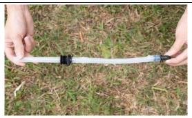
The peristaltic pump tube with no abnormality should be properly lubricated with the synchronizing plate. If the lubrication is poor, plain Vaseline or petroleum jelly should be applied.
