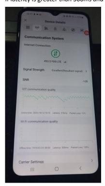
If using duo channel (WIFI/ 4G), please check both IOT and WIFI communication quality. The UAV will decide to use the channel that has the lowest latency and packet loss.
