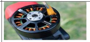
5. Motor Wire Inspection: Check whether the three-phase wires and terminals of the motor are worn or broken. It is necessary to wrap the three-phase wires of the motor with Acetate Cloth Electrical tape to ensure that the wire shielding is not exposed. Replace any motors with damaged wires or terminals.
