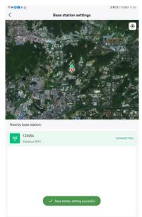
10. Wait for 30 seconds for RTK positioning to be active.
