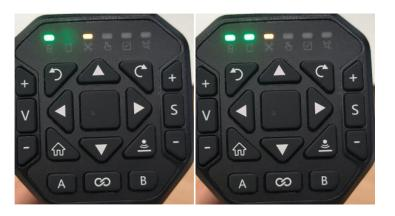
3rd led Flashing yellow: pairing mode or connecting to local wifi
