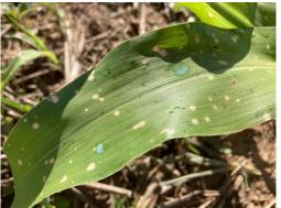
[velocity 8m/s, 8L/ha, spray width 6.5m, height 3m, droplet size 80rm]
