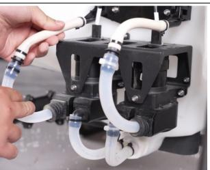
7. Check Hose Manually and visually inspect hose to check whether it is broken or worn.
