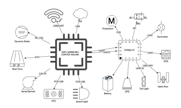
The real-time control unit and spray & spreader control unit adopt STM32H743 M7 core processor made by ST. Its CPU clock speed can reach up to 400MHz, 2MB maximum Flash, 1MB RAM; The positioning navigation unit adopts UM982, equipped with a three-axis accelerometer and gyroscope, barometer that can be auxiliary height measurement sensor.
