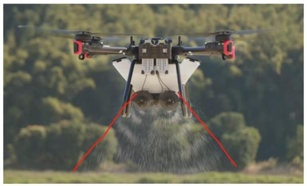
Two spreader disc is installed vertically. Spreader disc can apply force on granules, so that granules can reach the speed above 20m/s. Assumed the flight height is 6 meters, the spreader disc can shoot the granules onto the ground surface within 0.3 second. Benefit from this short of time, RevoCast spreading can eliminate the granules misplacement due to wind.
