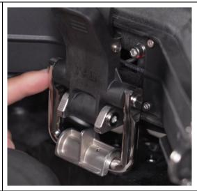
7. Inspect cable connector from loosening, eroding, deforming
