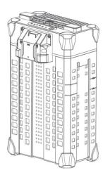
B13960S is the smart battery that has 13 lithium packs, with approximately 960Ah.
