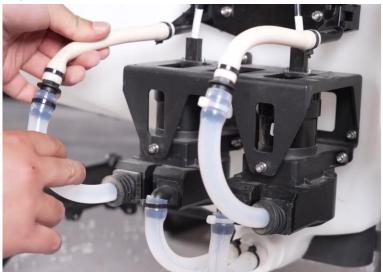
Remove the filter underneath the liquid tank
