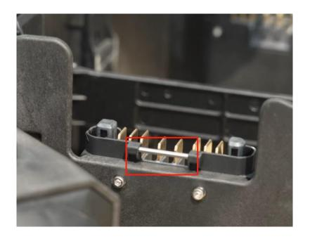
Make sure you hear the clip sound when plugging the battery socket
