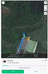
13 Mission completed. The UAV will turn off the spray immediately and ready to return the takeoff point.
