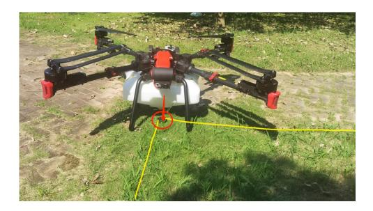
2. Go to the operation page and select the field you are going to work on, you will find the UAV symbol is not exactly at the corner. There is a deviation from the point where it should be and you are required to perform offset correction. Tap "Offset correction" button on the screen
