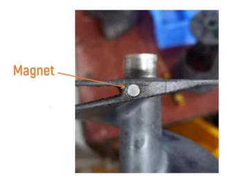
If magnet is loss, the spiral feeder will no longer work and need to be replaced.
