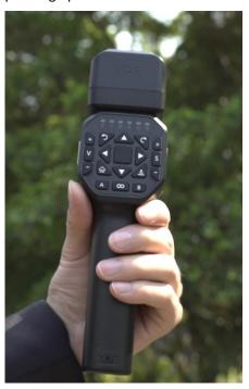
4. Walk into the field and add points. Press A to add points, Press B to delete points. \
