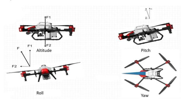
If the tilt angle reaches its limit, the UAV may lost balance and possibly crash immediately. To avoid this accident, please do not fly your drone when,
