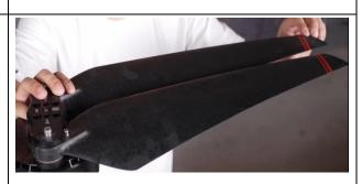
2. Check Propeller adaptor: Rotate the propellers horizontally to the limit position of the propeller adapter and check whether the limit position is misshapen or broken.
