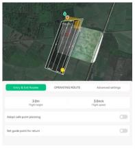
Operating Route (Fight Height, Flight Speed, Route Direction, Route interval, Boundary Safety Distance, Obstacle Safety Distance)
