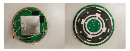
The bottom and upper view of main board with RTK module
