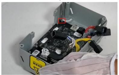
Step 2: Remove the mainboard and slowly buckle up both ends of the power board with two fingers. Naturally separate the power board from the head shell from top to bottom.
