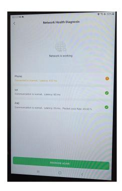
If network diagnosis fails, you will usually see the errors of IOT communication failures along with permission denied. In this case, you can remove all the devices from your account or consult with XAG technical support.
