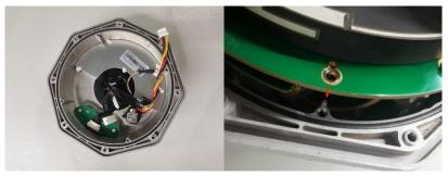
6. Remove GNSS antenna, unscrew 3 screws, unplug RF connector pin
