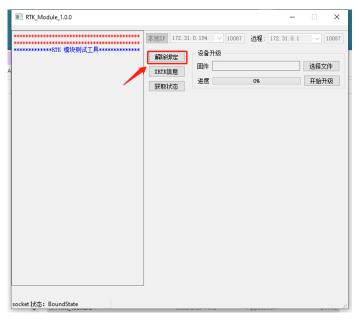
6. click the button XRTK 信息 (XRTK information) to obtain XRTK firmware version the XRTK information will display on the right the panel
