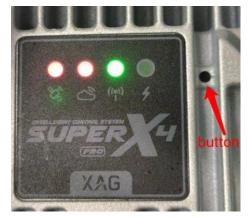
For P100H, release reset button of flight control when WiFi light indicator (the third light of flight control) alternates between green and red; Arm light slowly flashes yellow.
