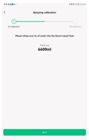
2. During spray calibration, the pump will deliver 6L water to the nozzle and the water will flow out of the UAV through nozzles. For the models before 2020, users were asked to place a measuring cup under the nozzle to know how much water was pumped by certain rotations of a pump. For the models after 2020, the liquid level sensor will measure and verify the volume of pumped water by itself.
