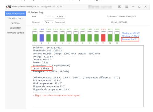
The below example shows the pressure difference is 117mV, which is not good. Please discharge and charge the battery twice and test again.
