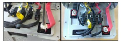
Step 2: Remove 2 cell sensor wires, 1 temperature sensor wire and 1 signal wire connecting the battery cell and BMS intelligent battery management system.
