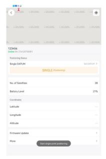
5. Once "FIX" is shown, the single point positioning is finalized Press "Save Coordinate"
