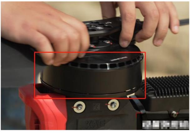
Rotate spray disk to check if the disk is firmly installed into the spray motor. Check if the spray disk can be rotated smoothly.
