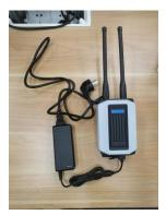
**Turn on LNT**: Long press power button for 2 seconds, release the power button when the  $1^{st}$  light indicator (Power) illuminates in green. Wait for 1 minute. The LNT is under initialization when  $2^{nd}$  /  $3^{rd}$  /  $4^{th}$  light indicators (WAN/WLAN/System) are flashing. Once all the light stop flashing and illuminate in green, the LNT is ready to use.
