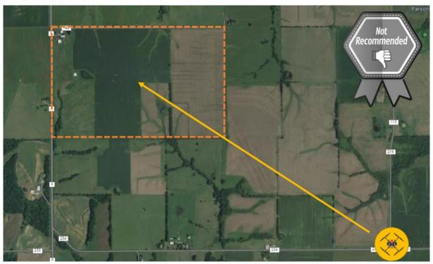
it's suggested to shorten the distance of entry and exit route. In this way, the drone can have more battery power in the field.
