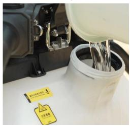
Make sure the remaining volume has enough liquid to perform manual spray test. You are allowed to set the individual pump flow rate and nozzle speed. The speed and current measurement of S1 and S2 should be very close.
