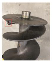
iii. Check if the magnet is eroded.
