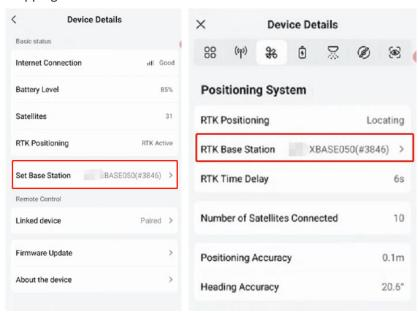
RTK fixed station has limited working coverage, normally 30km. Please make sure you are within 30km away from RTK fixed station.
