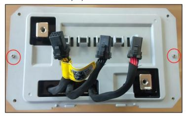
Step 2: Hold the lower shell with two hands, and the upper part of the shell contacts with the table. Lift the bottom of the shell upward to keep a certain angle to ensure that the battery pack can come out of the shell. When the external dimension of the shell can meet the holding distance, take out the battery with one hand and place it vertically.
