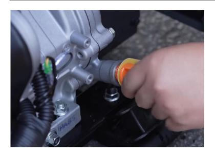
The  $1^{st}$  service should be taken placed after 20 accumulated operation hours. The  $2^{nd}$  and the reset of service should be taken place every 50 hours accumulated operation hours.
