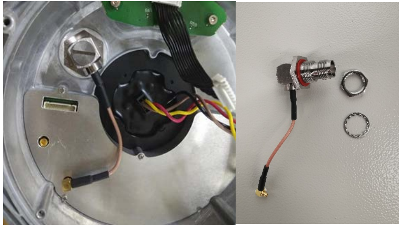
3. 02-001-03239, Fixture column waterproof gasket
