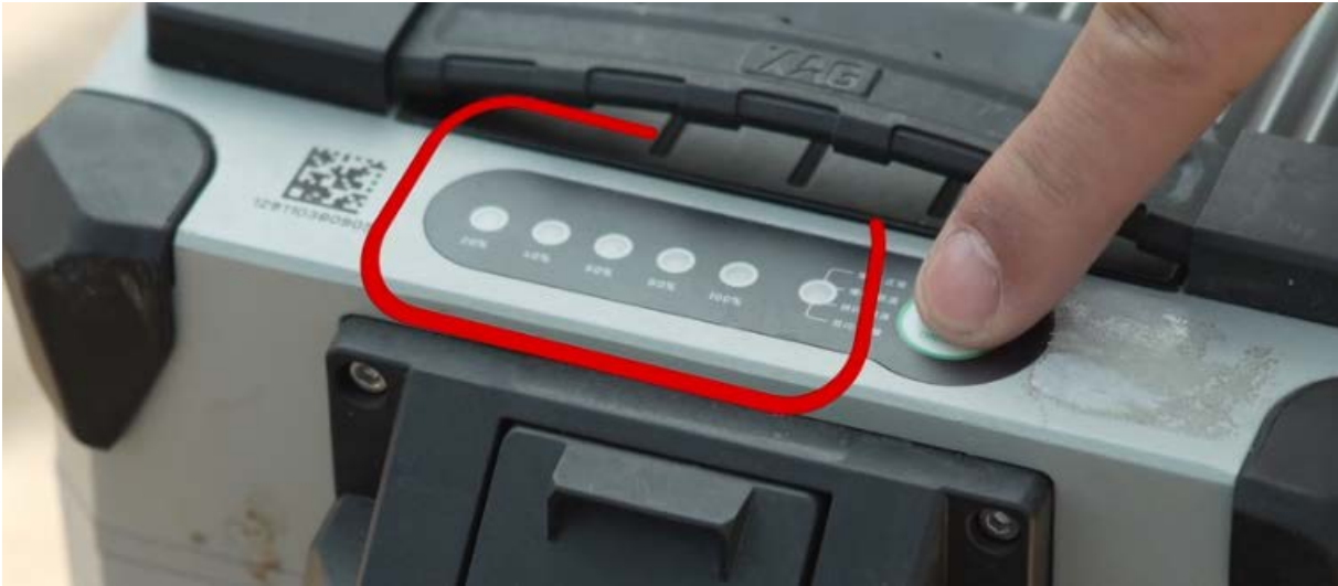
Check the remaining battery. Short press the smart battery power button
