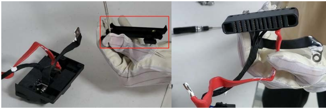
Step 2: Remove the battery plug case
