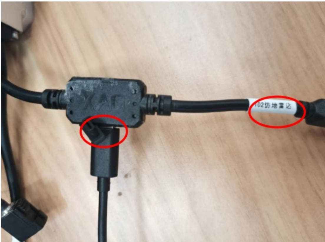
X4 PRO_LAN test cable connects 106 terrain radar to the computer network port.
