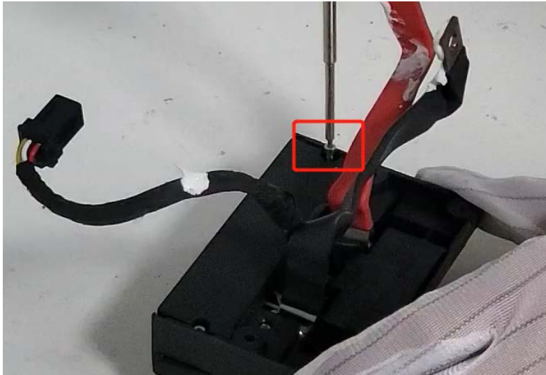
Step 2: Remove the battery plug case
