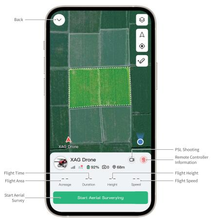
Back: tap to go back to the Field Page Flight Area: field area of aerial survey Flight Time: time for aerial survey Start Aerial Survey: tap to start aerial survey Flight Speed: flight speed during aerial survey Flight Height: height of aerial survey Remote Controller Information: view remote controller information PSL Shooting: namely "Pilot Sight Livestream", view current flight perspective of the aircraft
