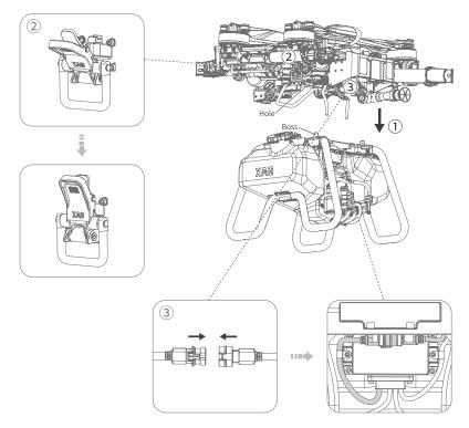
④ Connect the two liquid tubes to the pump of the RevoSpray system.
